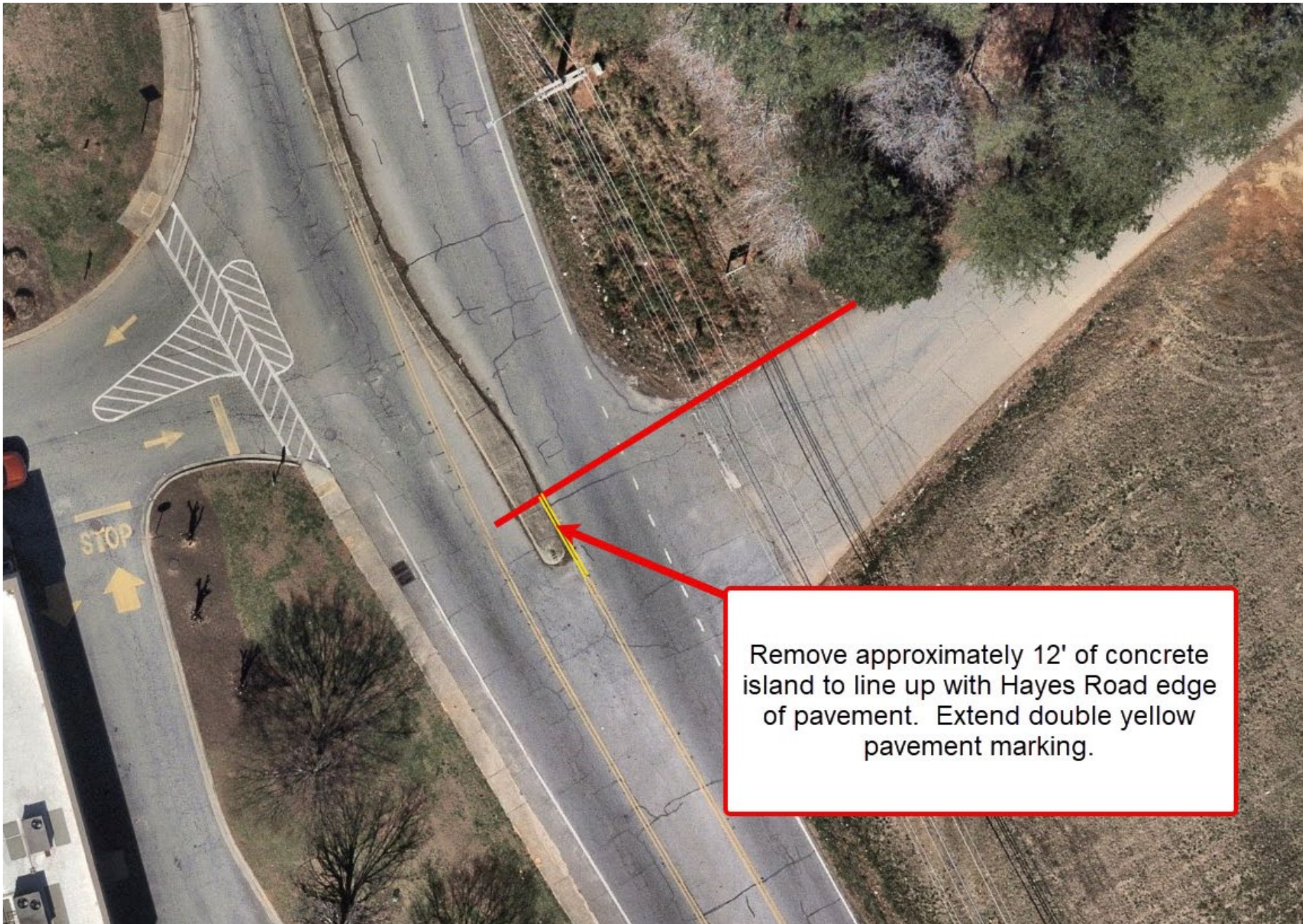
Figure 10. Concrete Island Modifications
