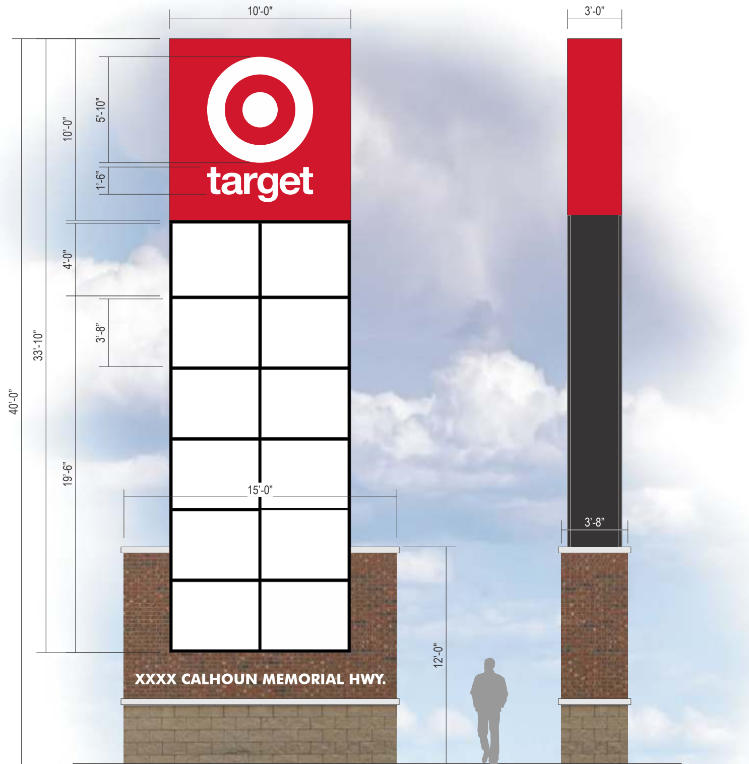
A D/F ILLUMINATED PYLON SIGN Scale: 3/16" = 1'-0"
