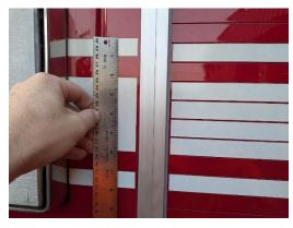
The front bumper shall have a 4" white retroreflective stripe for the entire length that is unobstructed by openings.
