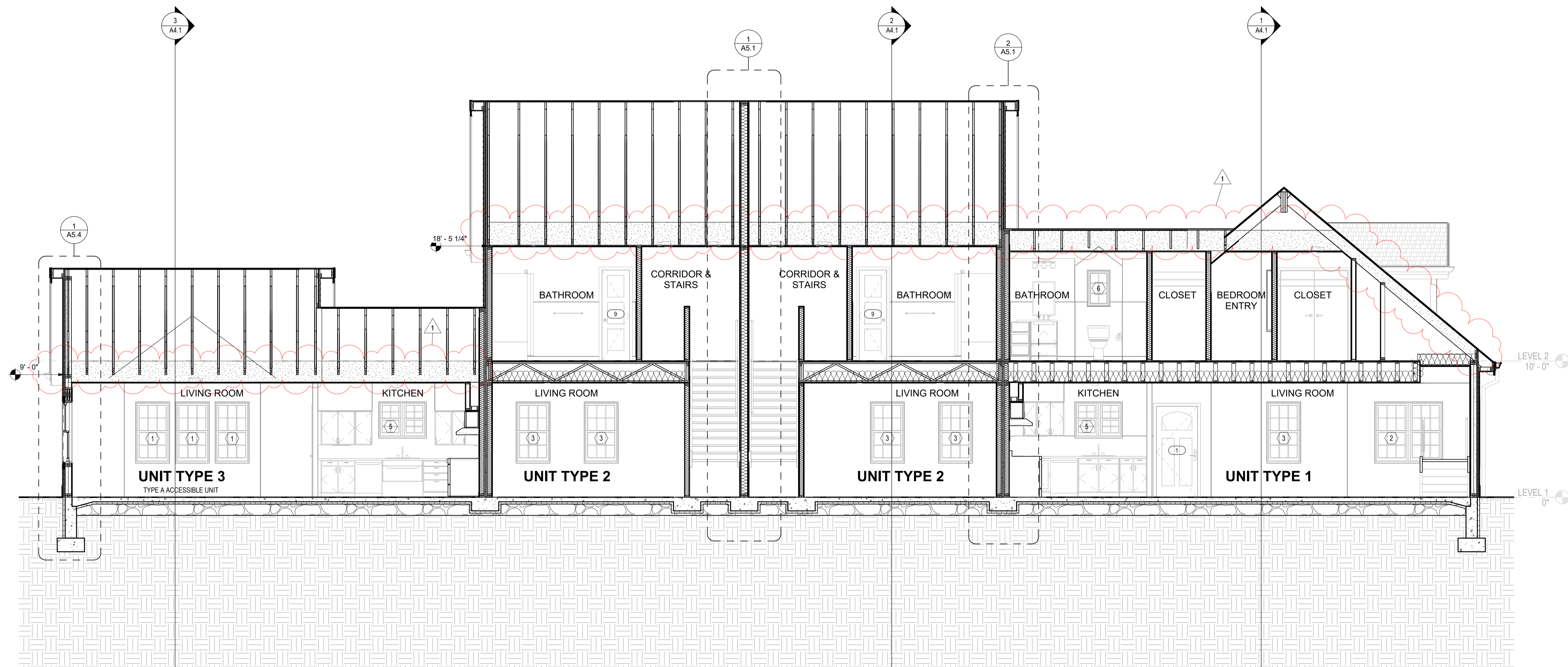
1 A4.0 OVERALL BUILDING SECTION 1/4" = 1'-0"
